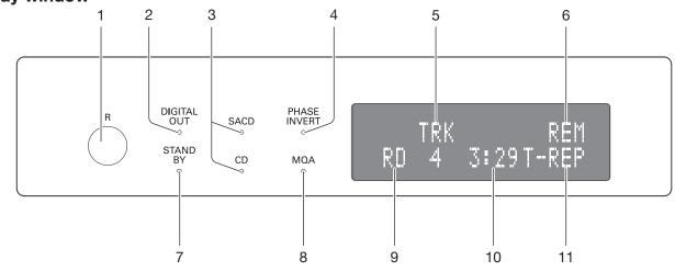
**1. Remote control infrared receiver (R)** Receives the infrared signals from the remote control.
